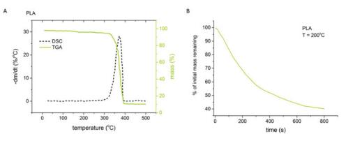
Figure 2. TGA and DTG analysis of PLA (A) and isothermal weight loss of PLA at 200°C (B). All measurements under nitrogen atmosphere. Initial mass 0.0502 g.
