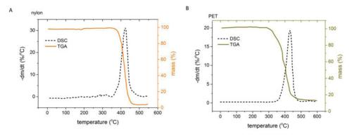
Figure 3. TGA and DTG analysis of nylon- initial mass 0.0499 g (A) and PET, initial mass 0.0510 g (B) under nitrogen atmosphere.
