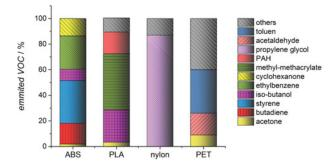
Figure 4. Emission of VOC during thermal treatment ABS, PLA, nylon, and PET. Results based on GS analysis.
